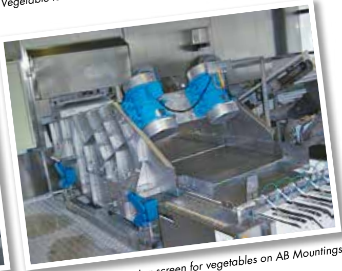
Vegetable-feeder on stainless steel ABI Mountings
