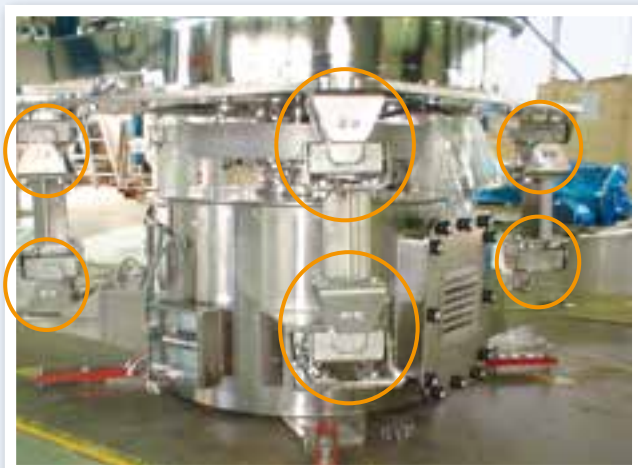
Gyratory screening machine installed on 8 pcs. AK-I 40 universal joints (joints made out of stainless steel)
