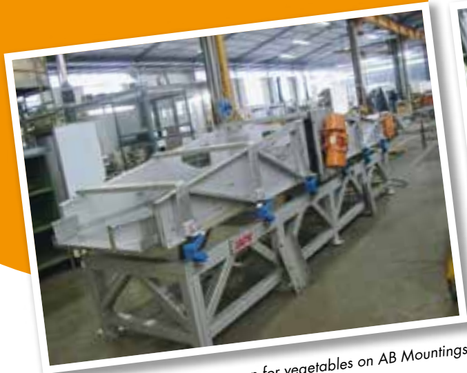
Vegetable-feeder on stainless steel ABI Mountings
